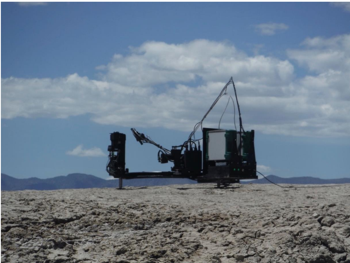
The RIT goniometer (GRIT) in the field. The GRIT instrument measures the spectral Bidirectional reflectance distribution function (BRDF) of natural surfaces at useful scales for supporting remote sensing science.
