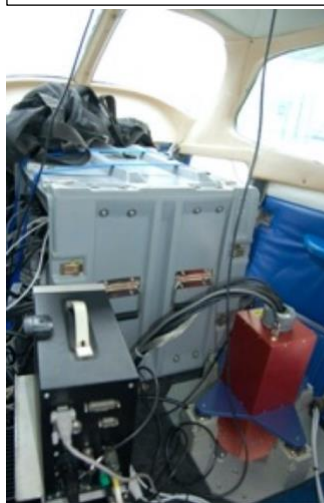
10-6. WASP lite in plane. The red box with blue mounting fins is the camera package (left) and view of cameras from below the plane (right).
