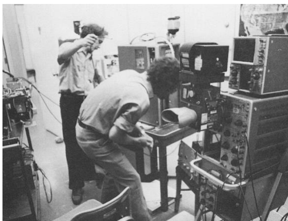
3-13. Gallagher (left) and Schott (right) with the tape recorder and film writing system. Note the oscilloscope viewer has a flip mirror to send the signal to the strip camera above and the conventional oscilloscope (top) is used to set up the Z axis (i.e. intensity) modulated oscilloscope.
