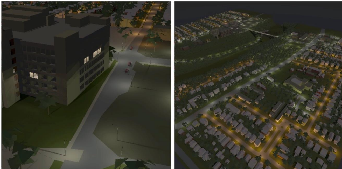
8-14. DIRSIG oblique nighttime “low light” camera image heavily contrast stretched to show scene detail (right). Note: the different color spectra from the tungsten, mercury and sodium lamps. The zoomed image at left shows another contrast stretched DIRSIG “low light” camera image of a portion of the Kodak Hawkeye plant where the light from fluorescent ceiling lights shows through the windows and allows some view into the building.
