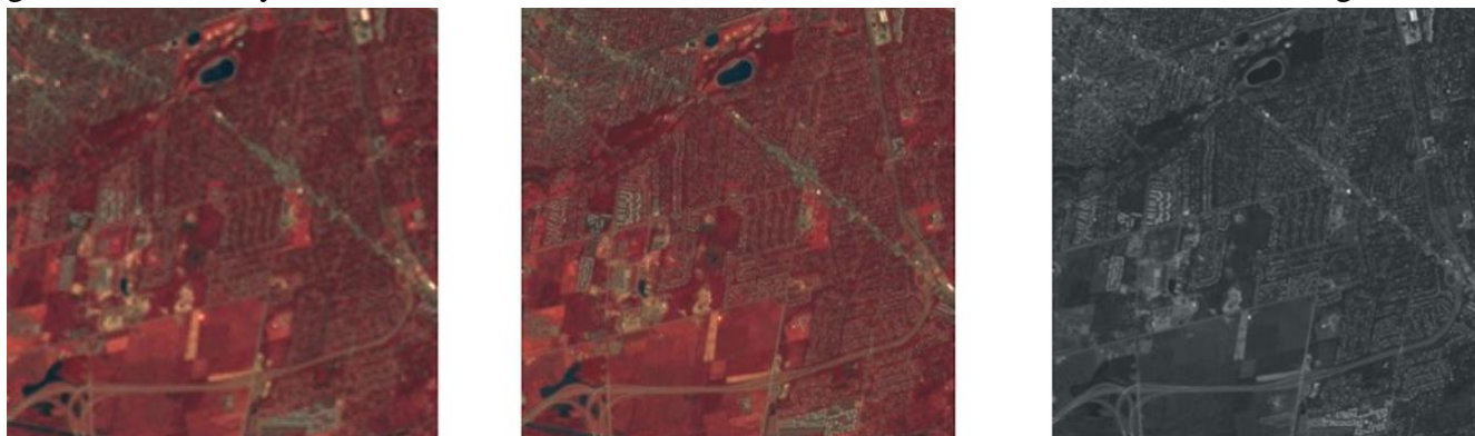
7-11. Left: Landsat color infrared image (30 m. pixels), Right: SPOT panchromatic image (10 m. pixels), Center: fused image combining the Landsat spectral data and the SPOT spatial data to form a 10 m. pixel sharpened color infrared image. This is one of many "sharpening" algorithms DIRS would develop for a number of sponsors.
