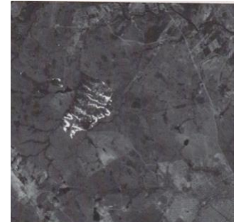
8-19. DIRSIG visible image of a grass fire at the edge of a forest canopy (left) and AVIRIS images of an actual fire in the blue region of the spectrum (center) showing smoke obscuration and in the short wave infrared (right) showing significant smoke penetration, raising the question of whether thermal infrared sensors are necessary for fire detection.
