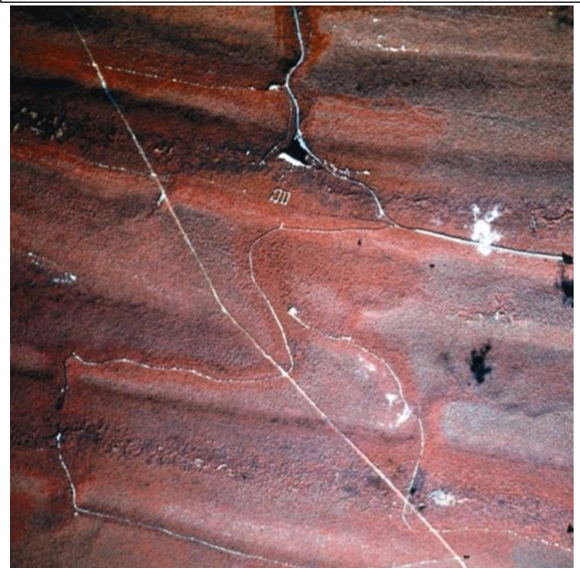
1-5. Color Infrared air photo of forested region in Pennsylvania with a gypsy moth infestation. Brighter red is indicative of healthier vegetation. Note, the effects of cosmetic spraying along roadways.
