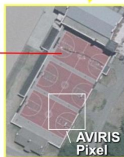
9-22. AVIRIS image of Lake Ontario shoreline (top left), invariant algorithm results (top right), spectrum of red paint supplied to the algorithm (bottom left), and aerial images showing the two targets detected and the size of an AVIRIS pixel indicating that the detections are subpixel.
