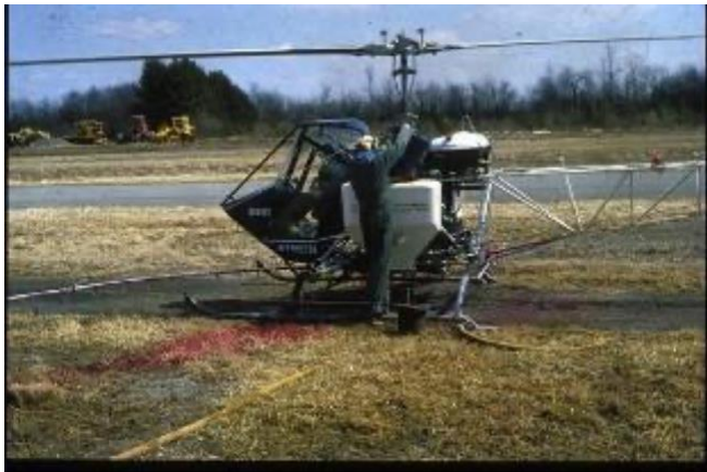
5-8. Spray chopper before taking off to mark ice on Lake Erie. Note: red stain from test spray under spray rig.
