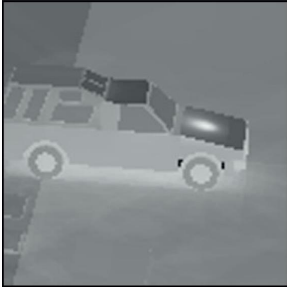
7-3. Early DIRSIG thermal infrared images showing the detail in the thermal and radiation physics incorporated even in the early versions of DIRSIG. The left image is a night time image. The thermal model "knows" the roof of the car will have radiantly cooled to the "cold" sky. It also "knows" the engine heats the hood above it. The sides of the vehicle are warmer than the top because they are in a radiational exchange partly with the cold sky and partly with the warmer ground. The pavement under the car is warm because it only "sees" the relatively warm car. The right image is a daytime thermal image showing how the shadow history that DIRSIG calculates feeds the thermal model which predicts that the grass in the sun will be cooler than the grass in the shade and that this effect will be quite quick (low thermal inertia) so the thermal shadows are relatively sharp. On the other-hand the concrete has very high thermal inertia so the thermal shadows take longer to form or fade as the solar shadow moves, resulting in much softer shadow edges and gradients away from the edge.
